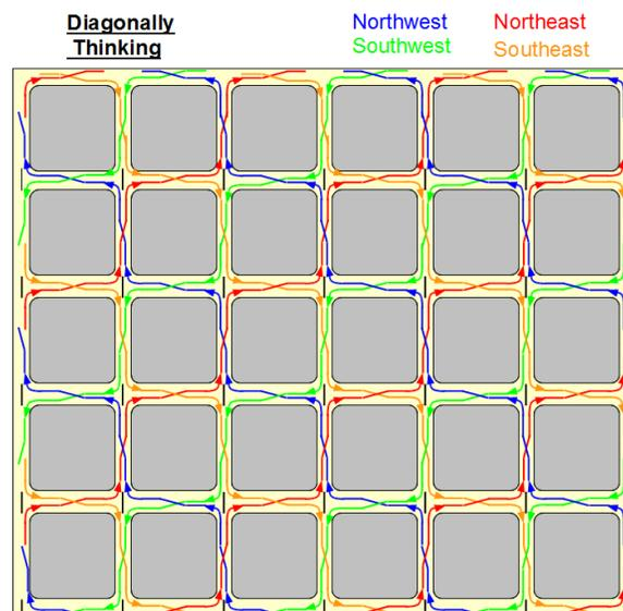
Note that we have implemented a 2D orthogonal diagonal grid, where each dimension is a set of interleaved one directional parallel paths. We have implemented it on a 2D orthogonal compass aligned grid. All streets in the compass aligned grid are one-way. All one-way streets have a length of only 1 block. All traffic splits left and right at the end of every block. There is no through traffic at any intersection. Every block starts with a merge.
